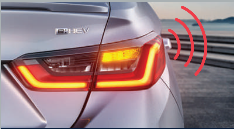
EMERGENCY STOP SIGNAL (ESS)
